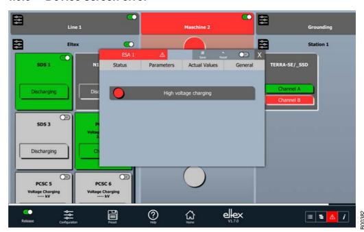
Fig. 18: Device screen Error
