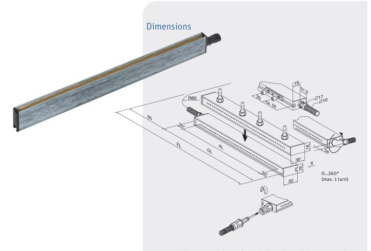
Overview and dimensions of the R50/R51A discharge bar and the L50 air profil EL = Installation length, AL = active length, GL = total length
